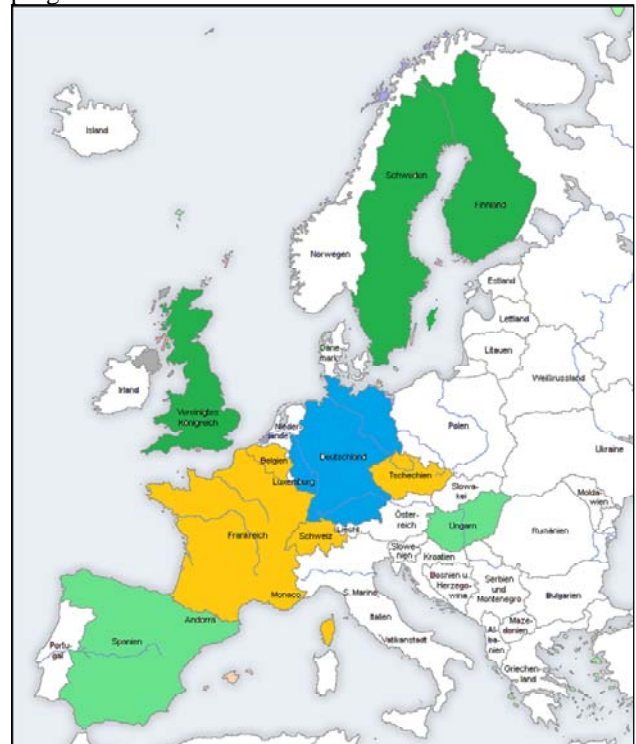
Fig.1: Preferential host rocks in the EU countries. green: granite, orange: clay, blue: rocksalt
